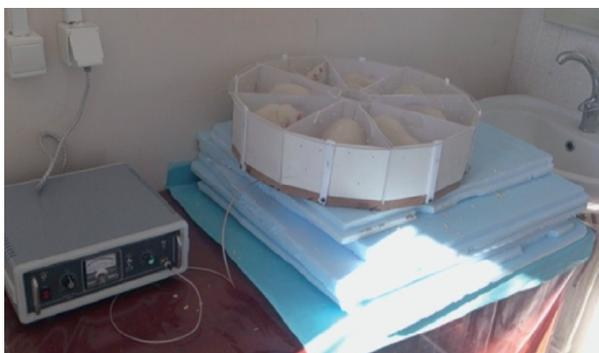
Figure 1. Magnetic field exposure apparatus
